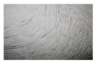
Grain flow is the directional orientation of metal grains resulting from plastic deformation during the forging process. Individual grains are elongated in the direction of deformation. While the strength and hardness of an alloy are a function of composition and heat treatment, fatigue strength, impact toughness and ductility can be significantly improved by identifying the critical loading locations of the component and ensuring that the grain flow is properly aligned.
